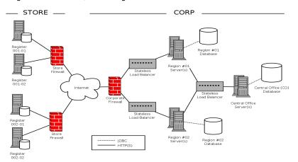
Each Regional database supports multiple stores and allows the network of nodes to scale. Asynchronous replication uses minimal bandwidth and handles periods of disconnected operation. Replication is configurable for one or both directions and includes conflict detection and resolution.
